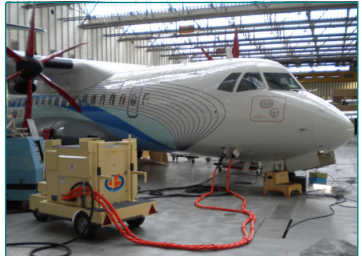
ABLE80 60KVA + 600A on heavy duty trailer.
