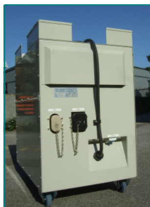
Aircraft connectors may be panel mounted on the GPU.
